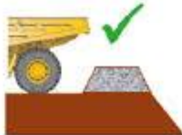
SUITABLE EDGE PROTECTION BERM PROFILE
