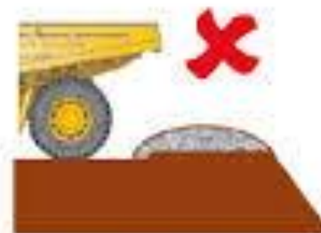
UNSUITABLE EDGE PROTECTION BERM PROFILE
