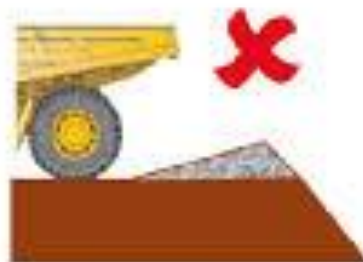
UNSUITABLE EDGE PROTECTION BERM PROFILE
