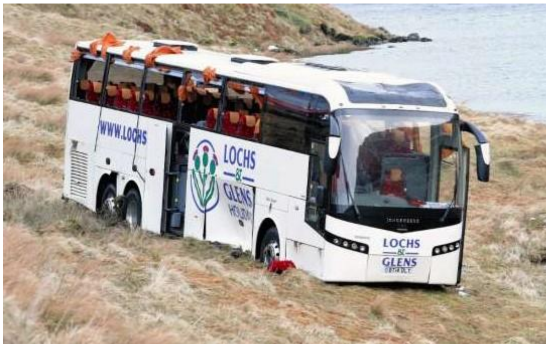
Photograph 5: The coach in its rest position after rolling 360° down the embankment
